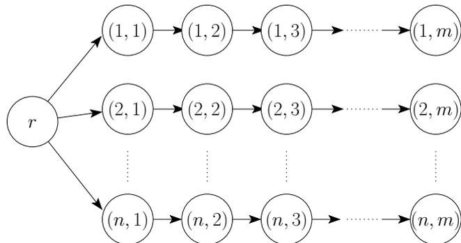
$$w((i, j - 1), (i, j)) = 1 + \left\lfloor 100 \left( 1 + \frac{j}{m} \times \left( \frac{n \times u_{i \times m + j}}{64007} - 1 \right) \right) \right\rfloor$$
